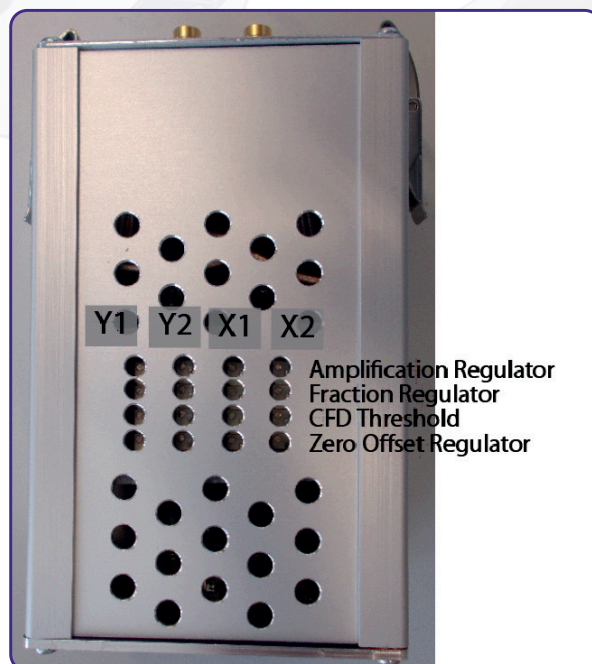
Figure 13: Labeling of discriminator threshold and amplification regulators.
